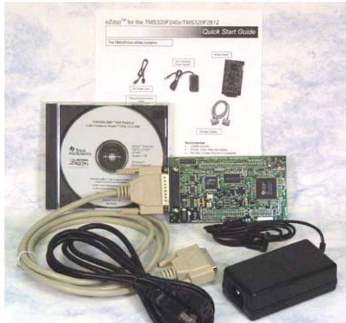
Figure 5: Spectrum Digital F2812 eZdsp Development Kit
