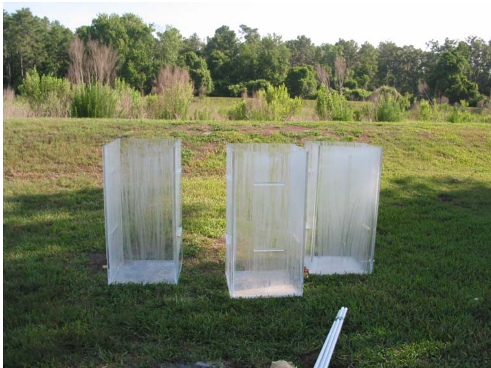
Figure 7 - Plexiglas Chambers at installation site
