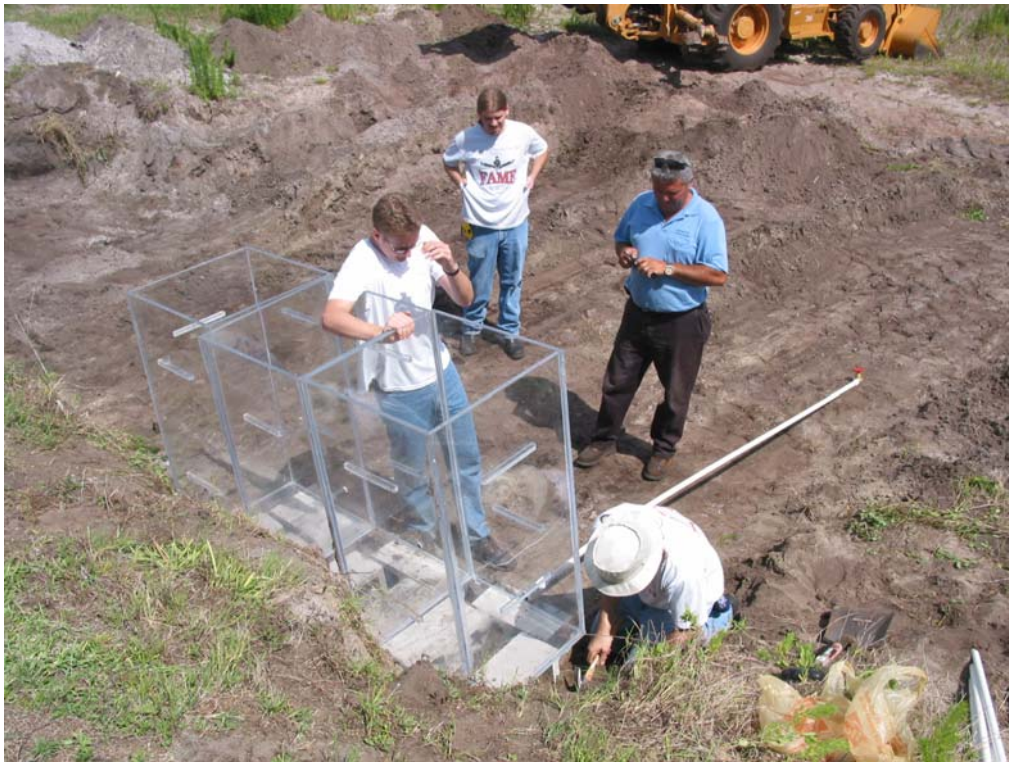
Figure 8 - Chambers are leveled
