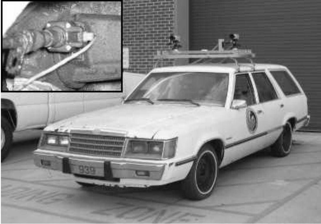
Figure 41 – 1984 FORD LTD Station Wagon Used for Mobile Platform, Vehicle Speed Sensor Attached to Transmission Shown in Inset.
