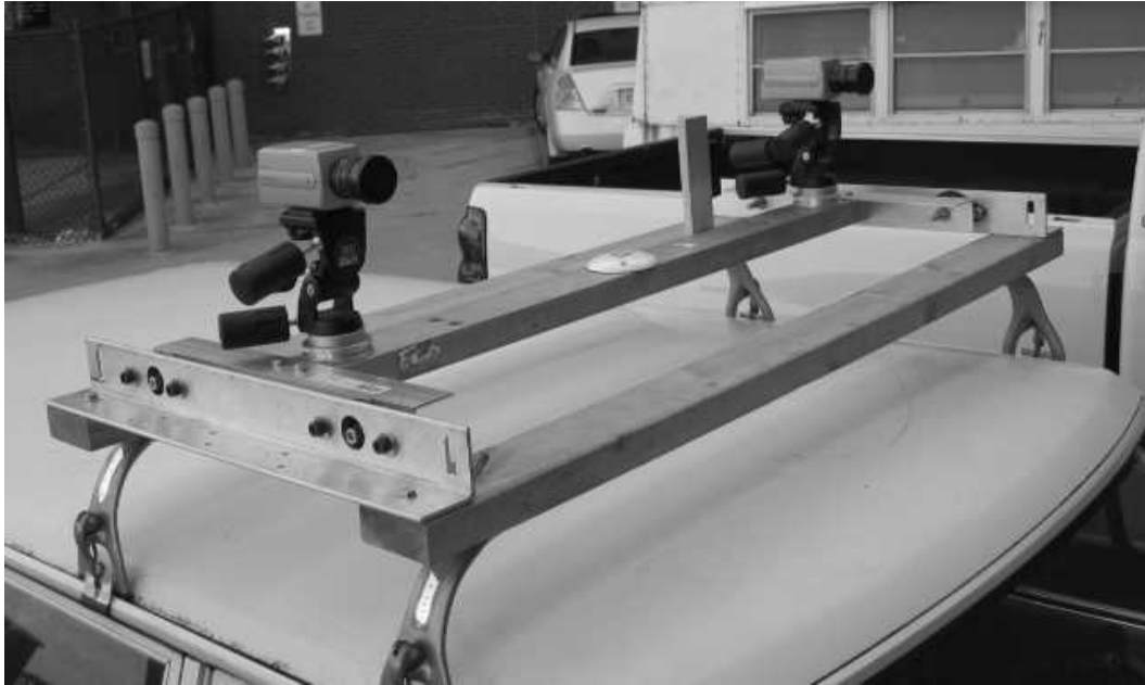
Figure 42 – Roof Mounted Carrier for Cameras, GPS Antenna and Compass
