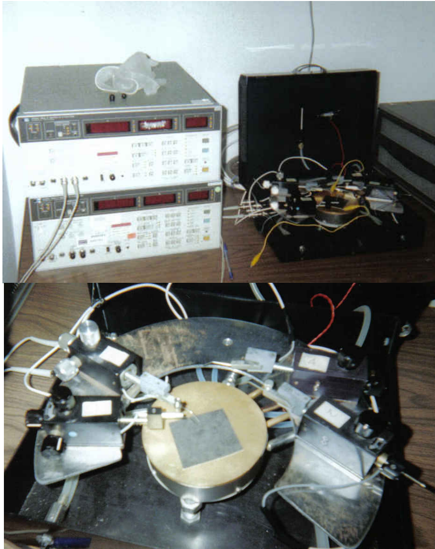
Figure 11: C-V Plotter used in this experiment along with the Signatone probe station with four probe tips.
