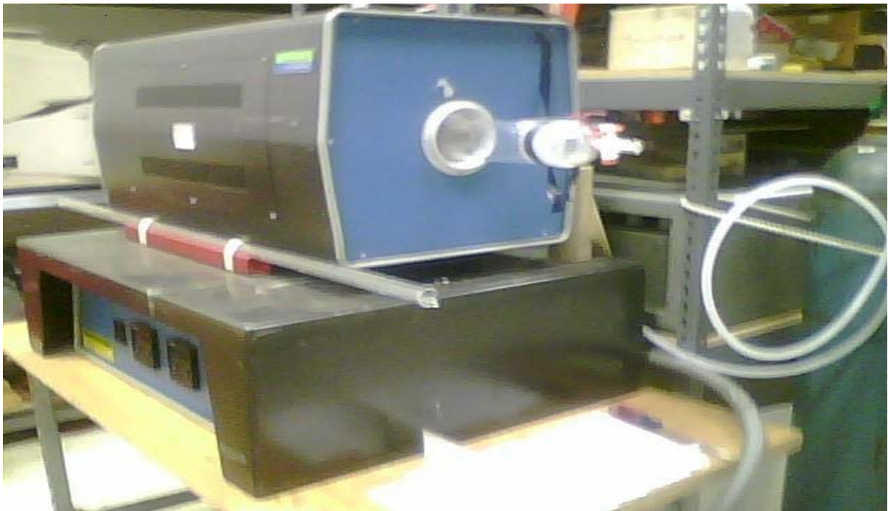
Figure 14: This is the oxygen furnace used for annealing made by Lindberg.
