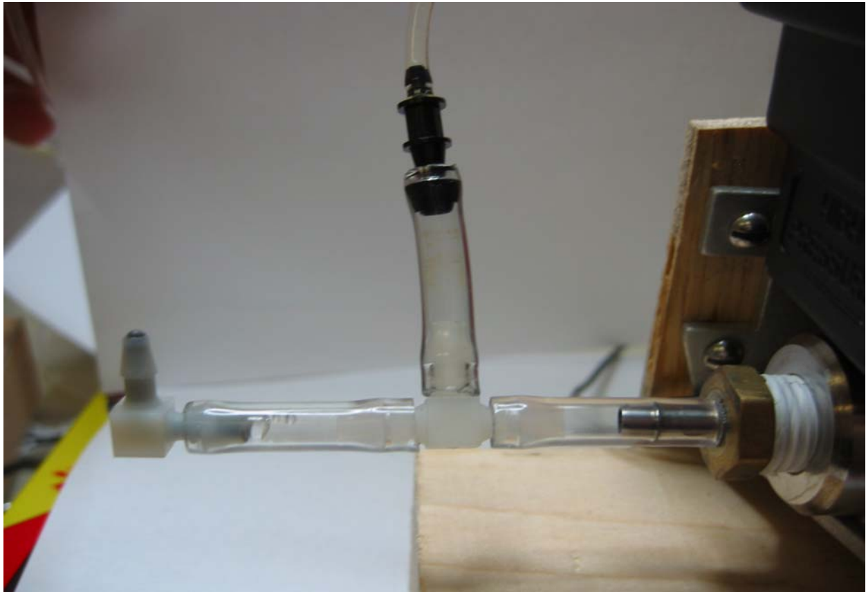
Figure 19: Flush plumbing for pressure port
