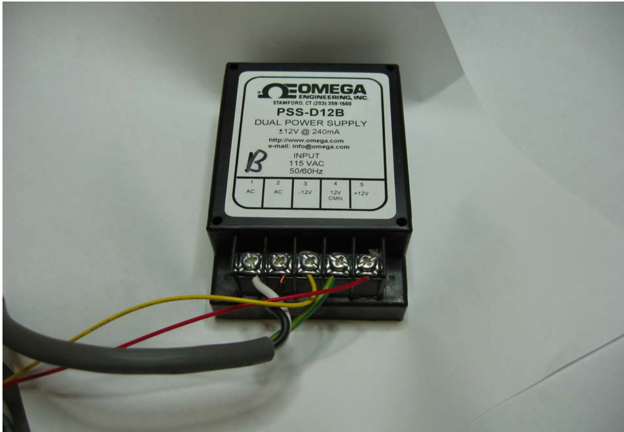
Figure 10: Transducer power supply
