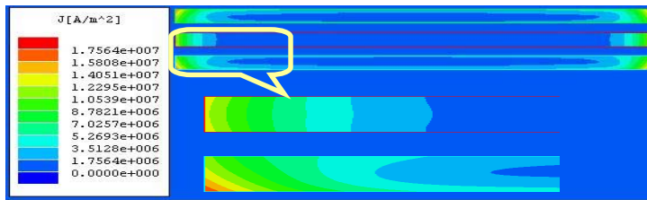
Figure 5-6. Proximity effect (three layers in parallel).
