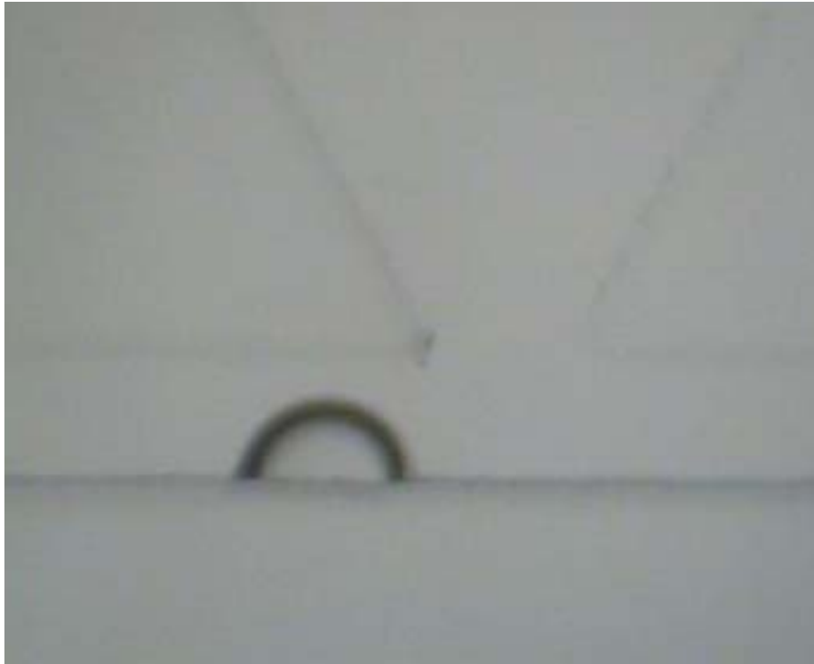
Figure 37: Bubble obstructing the flow in the test section.
