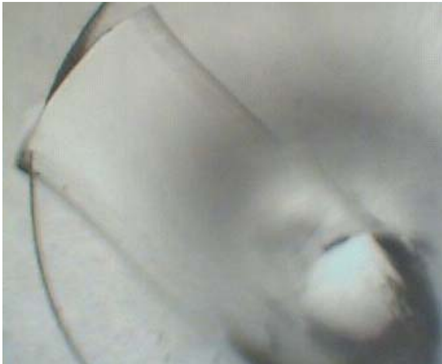
Figure 28: PDMS cylinder lodged into port.
