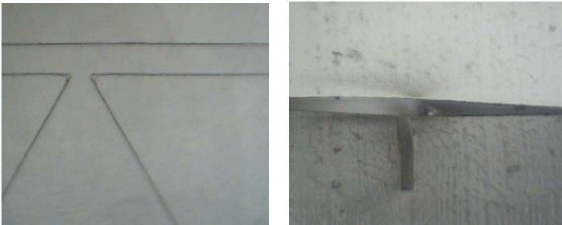
Figure 35: Channel leakage due to PDMS slab separation.
