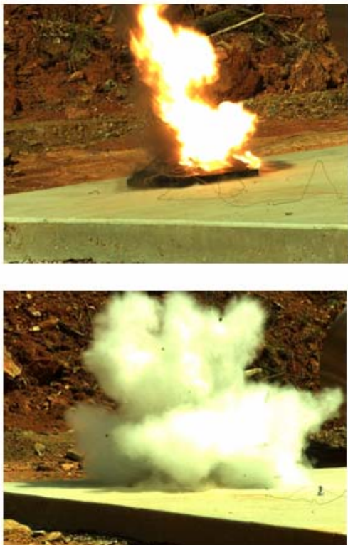
Figure 36: Pictures showing the comparison of the detonations of 2 grams of TATP (upper) and 88 g of TATP (lower)
