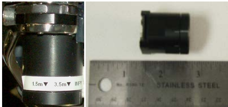
Figure 22: Monocular Lens-Mount Assembly.
