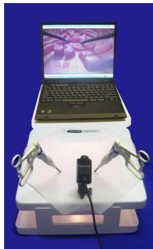
Figure 2 Laparoscopic Surgery Simulation Setup
