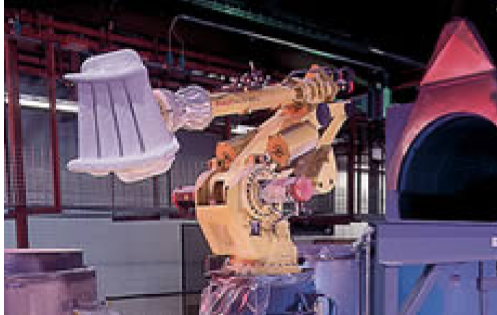
Figure 2.12. A robot dips a multi-stage vane segment at PCC Structural's Deer Creek facility (obtained from PCC Structural's (2009)).
