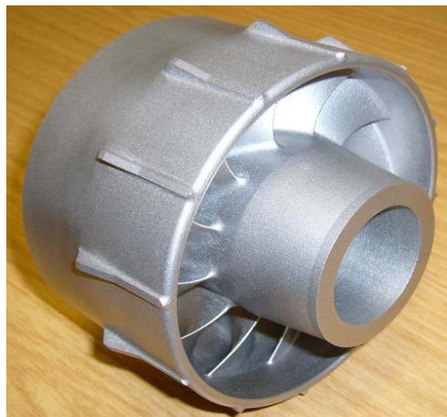
Figure 6.3. Air swirler created via DMLS using CoCr alloy.
