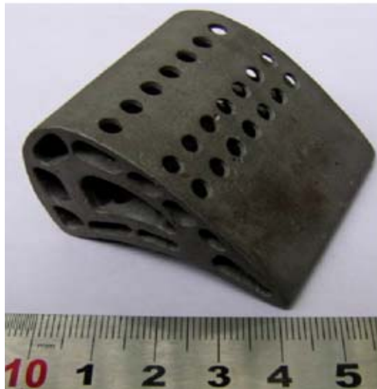
Figure 2.14. An investment-cast hollow turbine blade with cores removed (obtained from Wu et al. (2009)).
