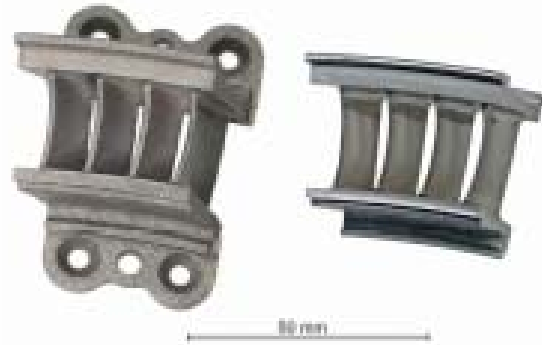
Figure 2.4. Vane segment in a nickel-base alloy as generated by SLM (left) and in the finished-machined condition (right) (obtained from Richter (2008)).
