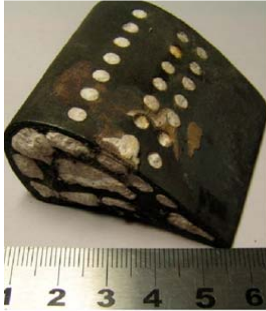
Figure 2.13. An investment-cast hollow turbine blade with cores (obtained from Wu et al. (2009)).
