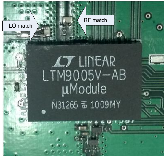
Figure 24: Integrated receiver subsystem. Matching is shown with the arrows.
