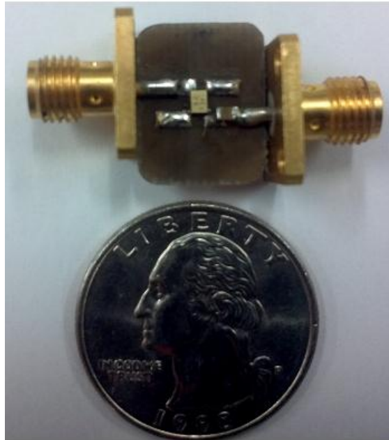
Figure 9: SAW ISM915 filter mounted on separate PCB. DC blocking capacitor added to protect miniature part from the DC voltage damage.
