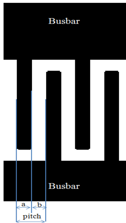
Figure 4-2 Zoom-in view of the 2 pair of eletrodes of the reference resonator
