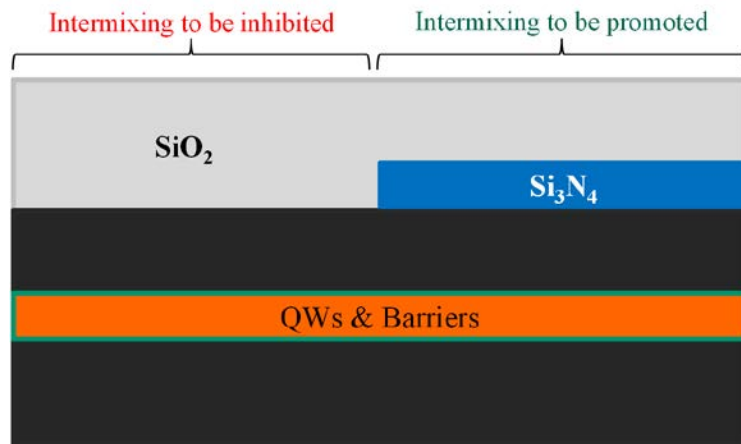
Figure 5-9. Schematic of dielectrics deposited selectively on quantum well sample to be able to define the regions that intermixing is needed to be promoted (SiN x capped) and inhibited (SiO 2 capped).
