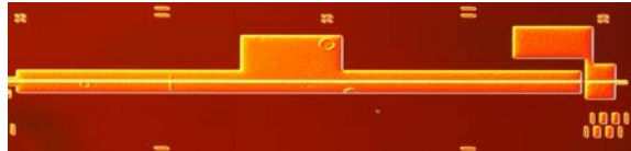
Figure 3-3. Top view image of the fabricated 2 mm two-section mode-locked laser
