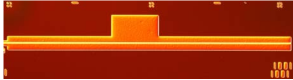
Figure 2-8. Top view image of the fabricated 2 mm Fabry-Perot laser device after p-contact annealing
