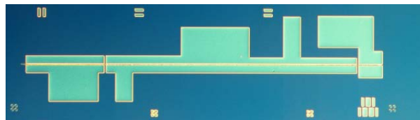
Figure 5-17. Top view image of the fabricated 1.9 mm three-section mode-locked laser
