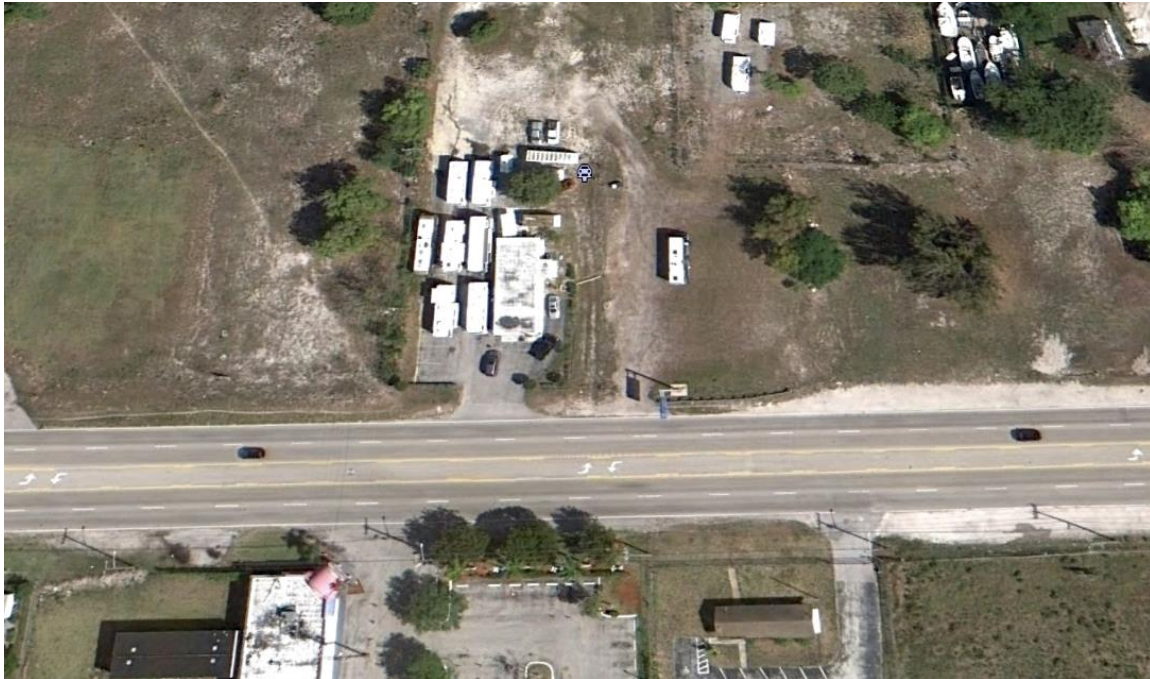
Figure 1-1: An Example of Two Way Left Turn Lane (TWLTL) Median (Source: Google Earth)
