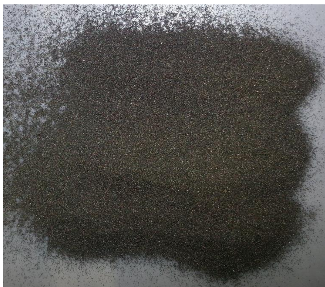
Figure 10: Image of Ni-185 and 2% wt CNT Mixture with PEG Binder
