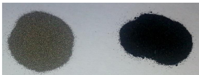
Figure 5: Stock Ni-185 (Left) and Jar Mixed Ni-185 & 1% wt EFGO (Right)
