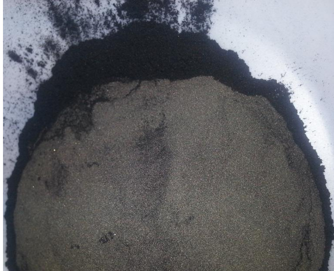
Figure 8: Photo of Ni-185 and 2% wt CNT after 8 Days Jar Mixing
