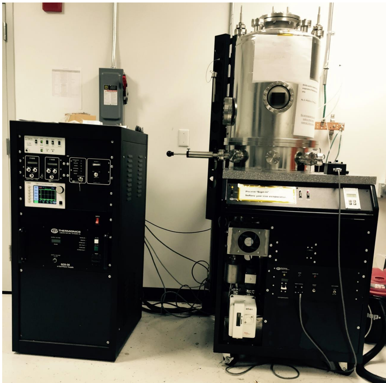
Figure 3.7 Actual image of thermal/e-beam evaporator used for deposition of Au NPs on flakes.
