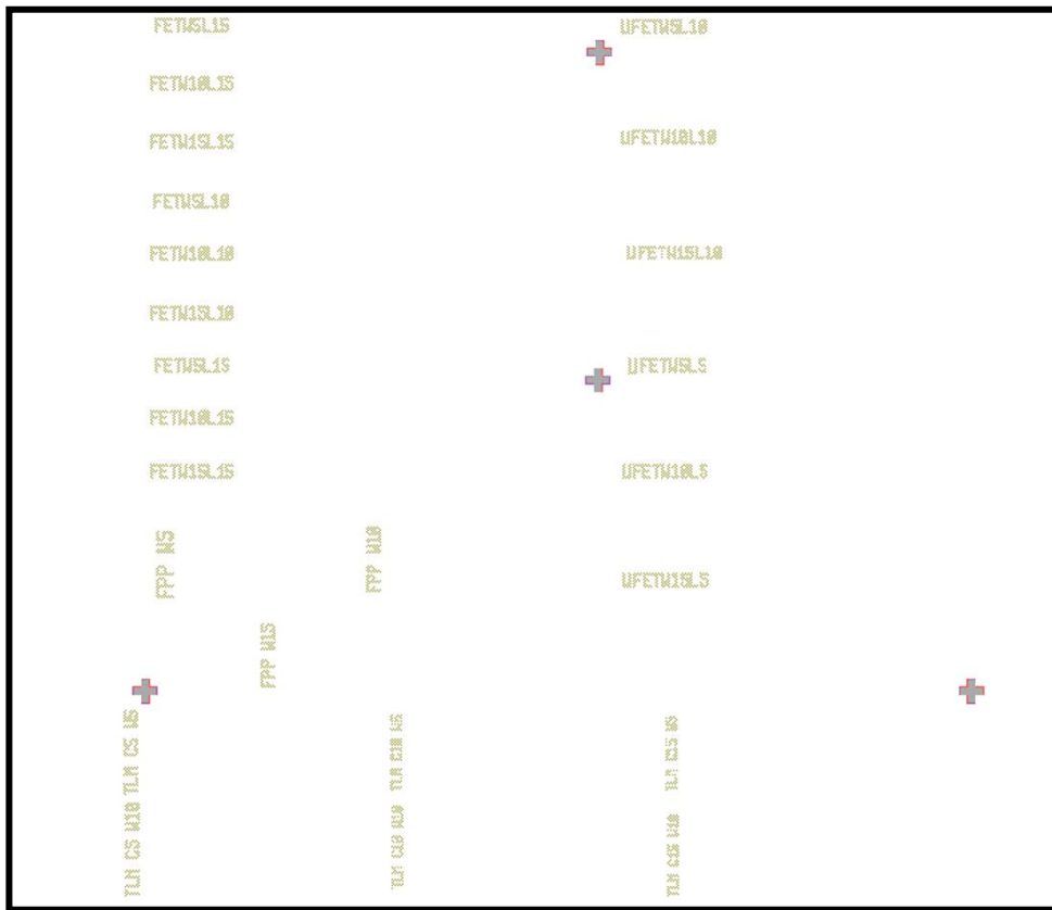
Figure 28. The first level mask used for patterning the alignment marks for fabricating the MoS 2 /graphene devices.
