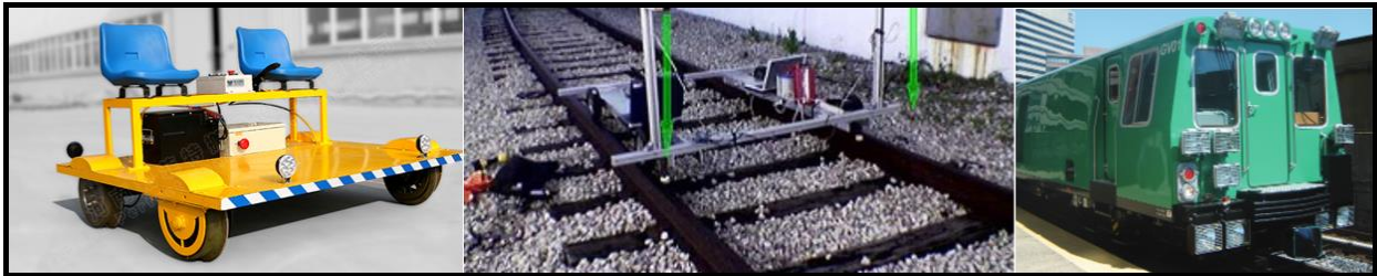
Figure 1 Various platforms for railroad inspection
