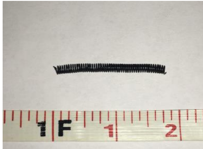
Figure 16 SMA spring as received from the manufacturer. This spring had not been tested on, thus is in its solid length pictured above.
