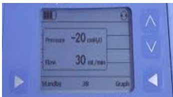
Figure 3. The monitor displays the suction amount and the air flow in the pleural space.
