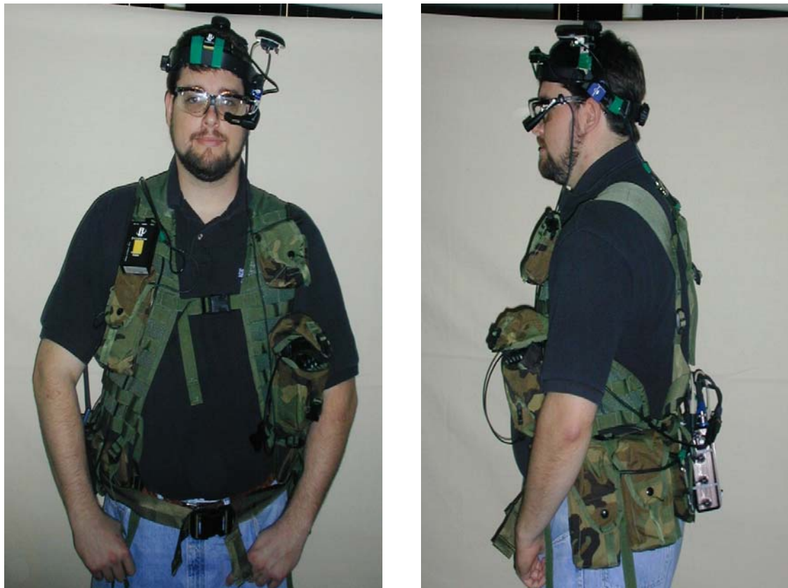
Figure 5: Front and side view of the battlefield augmented reality system (BARS)
