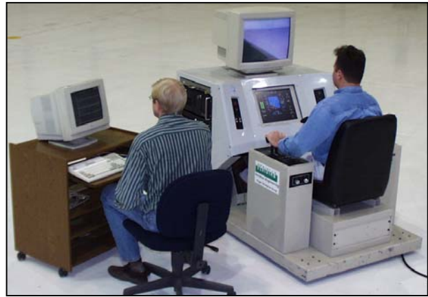
Companion Ground Trainer Used to Prepare Trainee for In-Flight Simulator Training
