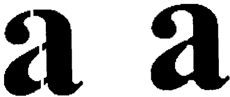
Figure 6: a) Broken Character; b) Restored Character by Closing Filter
