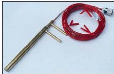
Figure 30: water-cooled Gardon gauge to withstand much higher heat flux levels.
