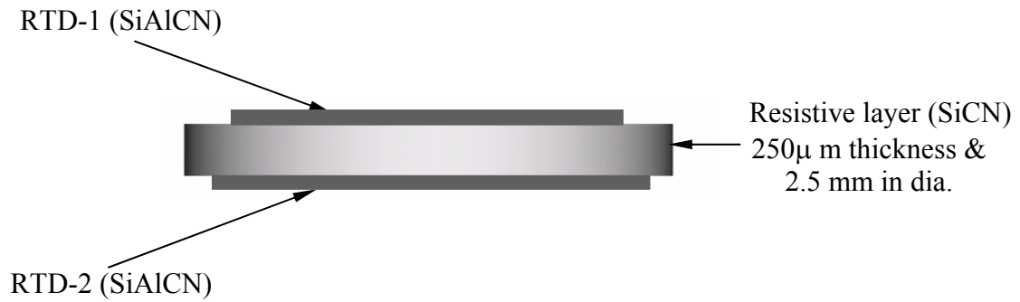
Figure 33: Side view of proposed heat flux sensor
