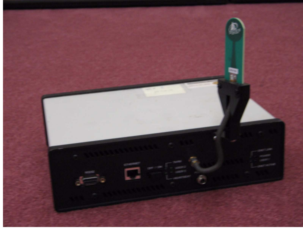
Figure 4.1: Time Domain P-200 radios used as the intruder detection sensor.
