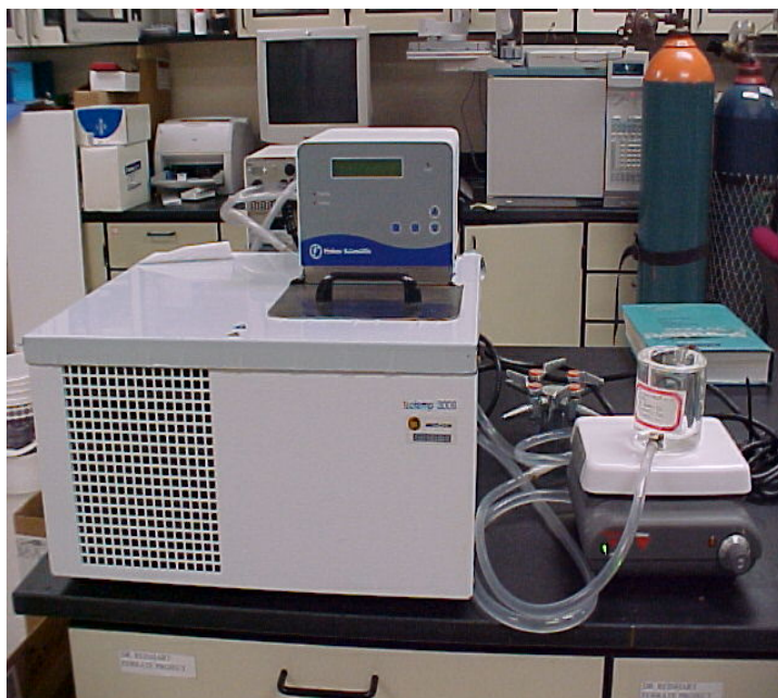
Figure 3-1. Bench-Scale Unit used for the Ferrate Preparation
