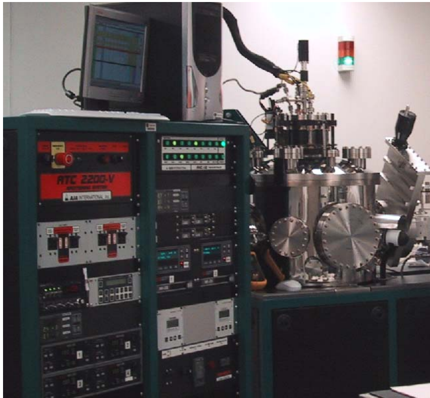
Figure 6: The AJA International sputter system used in this research.
