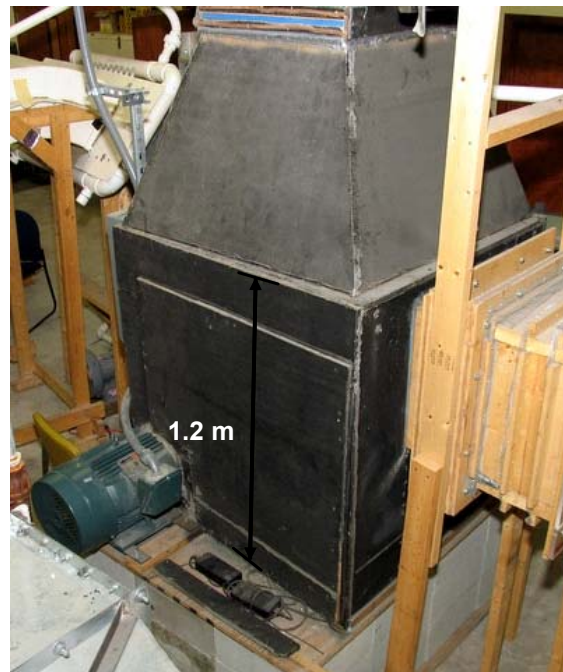
Figure 3-3 – Blower casing with motor
