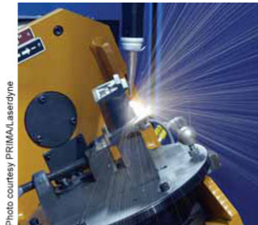
Figure 1-4 – A LASER drilling holes into a blade surface
