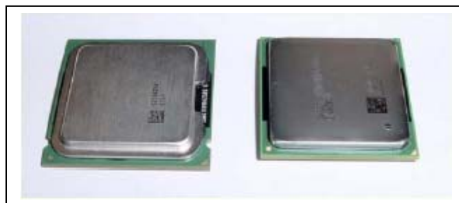
Figure 2.1.3 LGA 775 and mPGA 478 Packages
