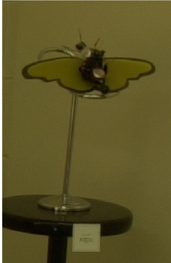
Figure 4: DiSection : The Second Interactive Creature. Designed to Arch and Bend in Response to Sound
