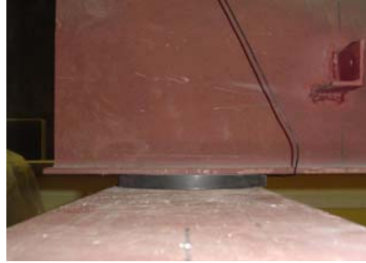
Figure 40: 1 Duro50 Pad Support (BC3a)
