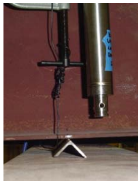
Figure 39: Pin Supports (BC1)
