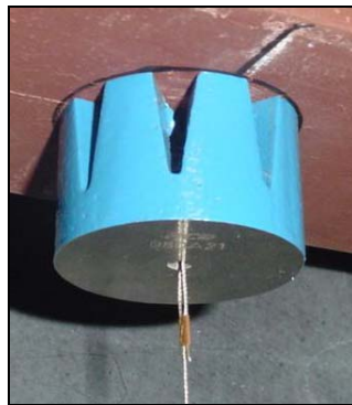
Figure 24: Displacement Cable Attachment Method
