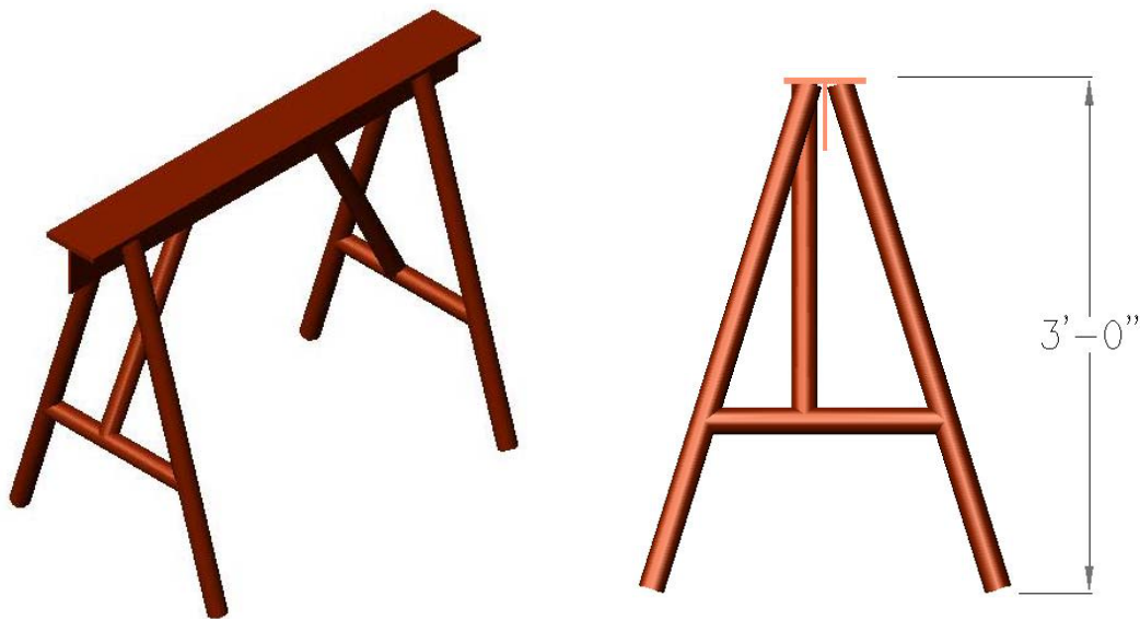
Figure 14: Test Beam Sawhorse Support
