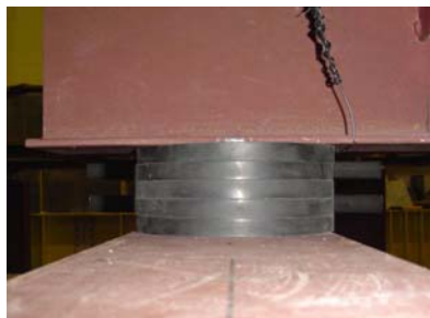
Figure 41: 5 Duro50 Pad Support (BC3b)
