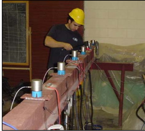
Figure 22: Impact Hammer Tests on the Beam
