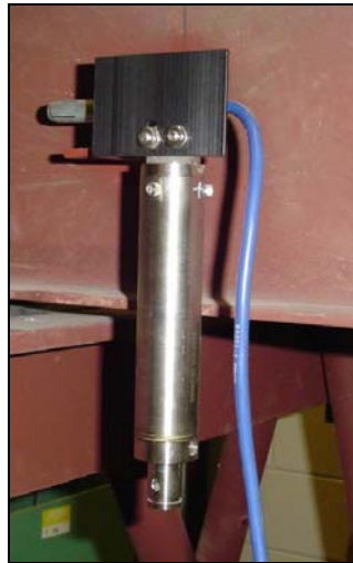
Figure 25: Geokon VBWG Tiltmeter
