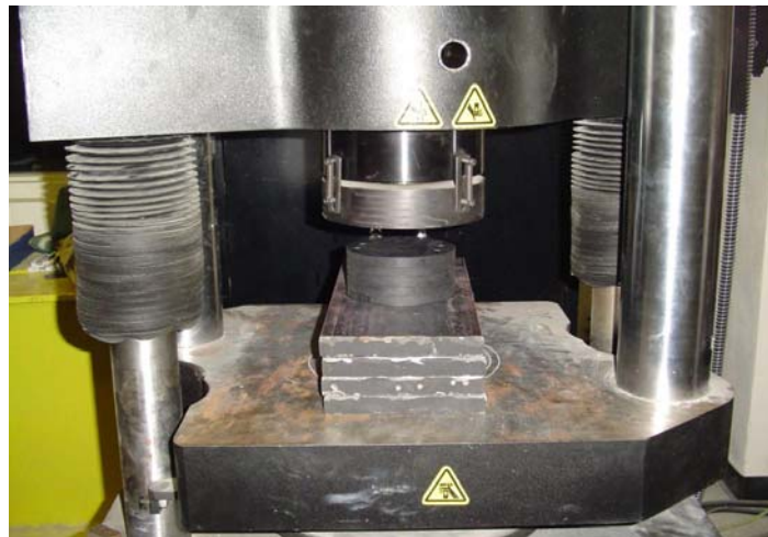
Figure 34: Compression Tests of 5 Duro50 Pads Using UTM
