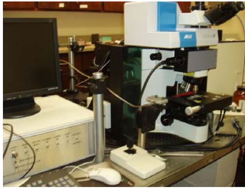
Figure 9: Front view of confocal Raman system and computer setup for control of system (viewing spectral data, camera viewing through microscope, and control of spectroscopy software)
