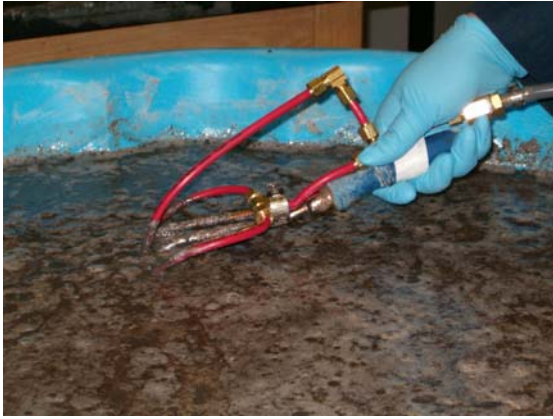
Figure 15 - Action of injected emulsion into sediment.
