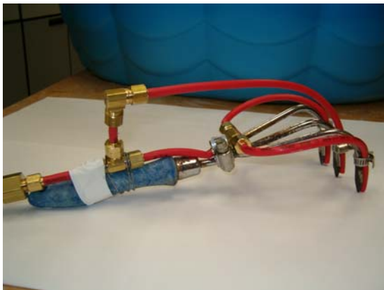
Figure 14 - Apparatus for injecting emulsion.
