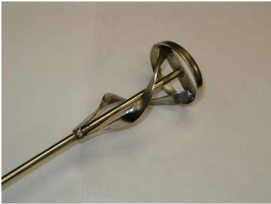
Figure 16 - Attachment for soil mixing.
