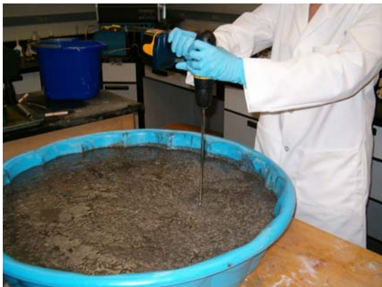
Figure 17 - Mixing of emulsion into sediment.
