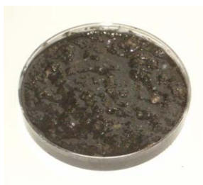
Figure 19 - Sediment mixed with microscale iron emulsion.
