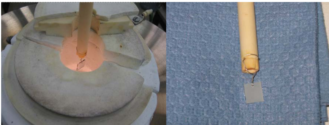
Figure11 Post growth view of vertical substrate settings.
