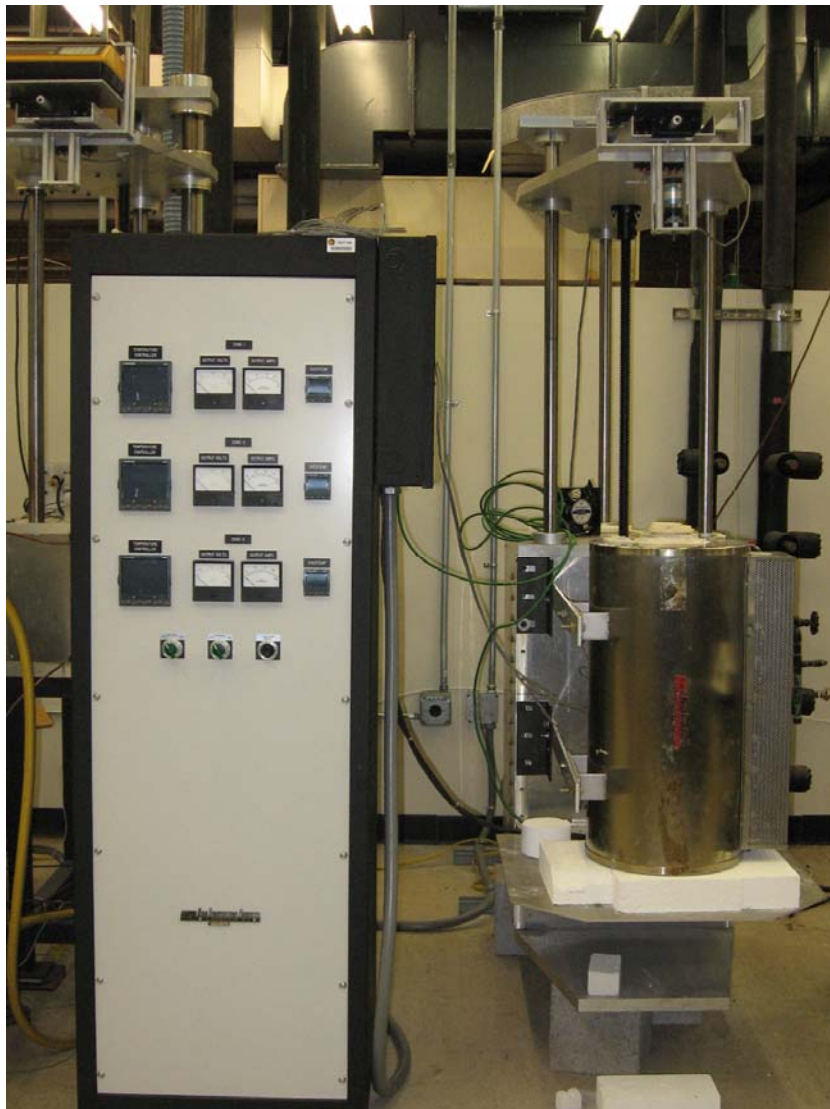
Figure 10 Picture of 3 zone Pt furnace LPE growth system
