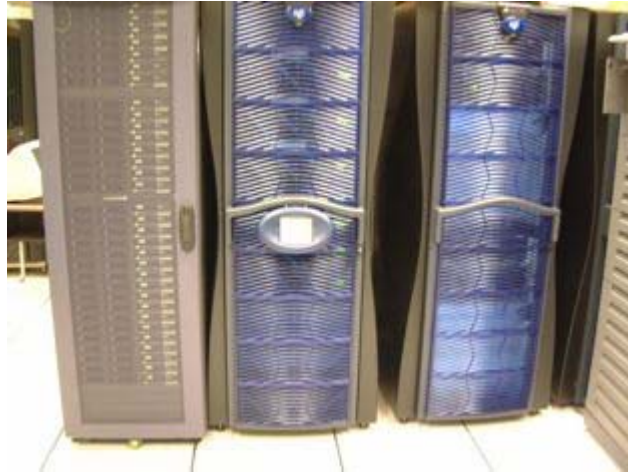
Figure 31. 48-node dual-processor Ariel Solaris cluster at UCF
