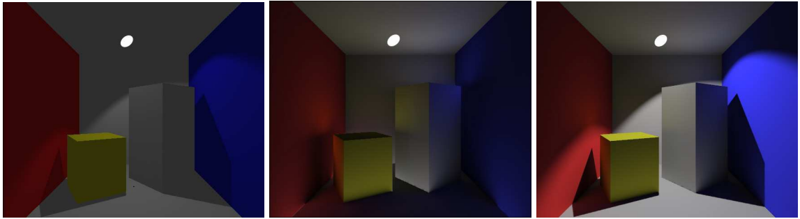
Figure 2.1: Global Illumination. (a) First evaluation (direct illumination) of the rendering equation in which only the light source emits light. (b) Second evaluation (indirect illumination) of the rendering equation in which the reflected light from the first evaluation is considered as incident light. (c) Final image rendered using both direct and indirect illumination. Images courtesy of Juraj Obert.
