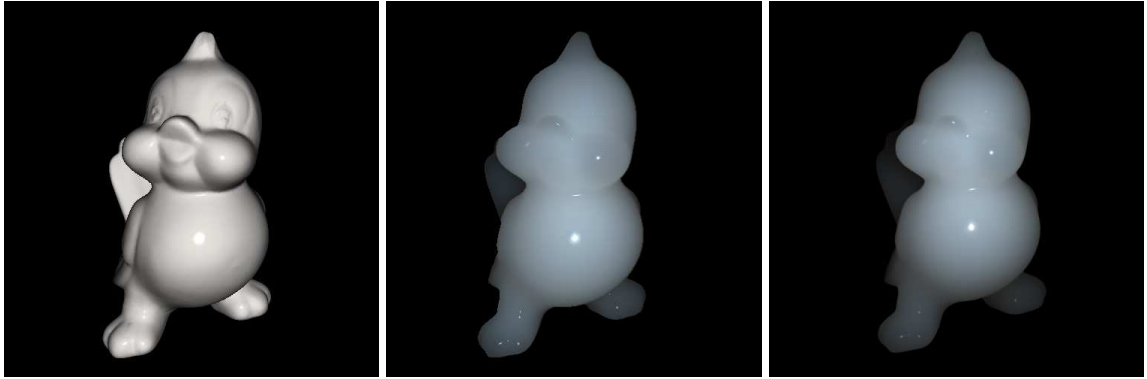
Figure 6.1: From left to right: bird model rendered (a) using Lambertian diffuse and Phong specular lighting, (b) our subsurface scattering algorithm (27 fps), and (c) an offline renderer (approx. 3 mins per frame). Note the translucency at the cheek and feet regions in the latter images.
