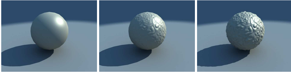
Figure 3.2: A sphere (left) rendering with bump mapping (center), and displacement mapping (right).
