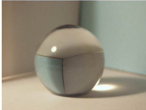
Figure 5.2: Photograph of caustics from a spherical glass paper weight using a desk lamp to emulate directional spotlighting. The caustics are formed on rough paper placed underneath the refractive object.
