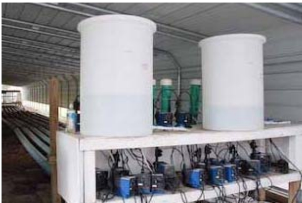
Figure 3-2 Influent Standpipes, Inhibitor Tanks and Pipes System
