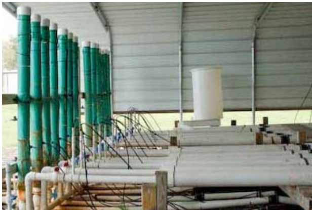
Figure 3-2 Influent Standpipes, Inhibitor Tanks and Pipes System
