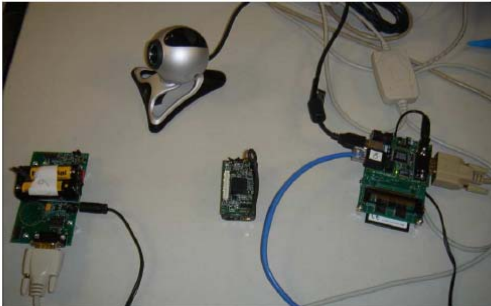
Figure 9: Sensor node data being collected by the central computer and the webcam
