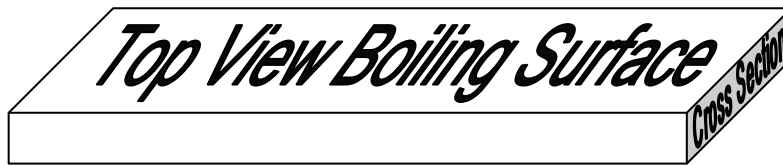
Figure 23: Schematic of view orientation of SEM and EDS analyses.
