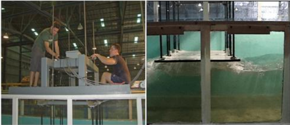
Figure 17: Left: Steel Support Structure for Models Right: Flat Plate Bridge Model during testing in wave basin tank. (Sheppard, 2009).
