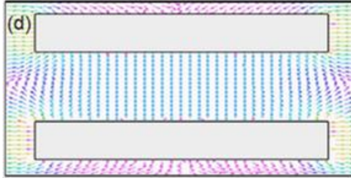
Figure 3-4 simulation of the electric field lines in between the two electrodes separated by 5 \mu\text{m} gap.
