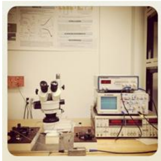
Figure 3-6 Actual setup for DEP to trap carbon nanotubes in between the electrodes.
