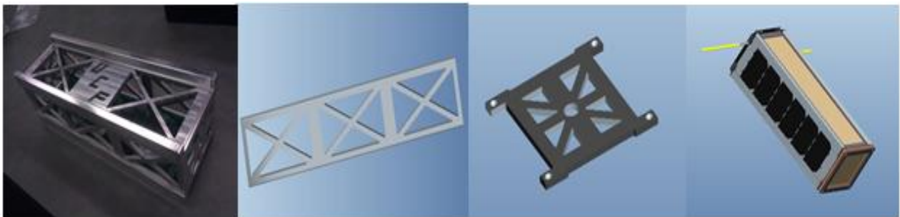
Figure 2: Fabricated Prototype, Side Panel, End Panel, Full Satellite with Solar Panel
