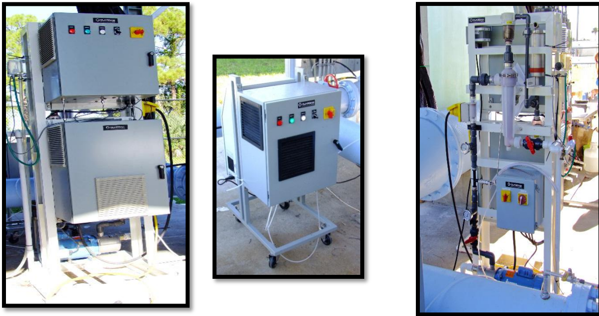
Figure 4-2: Ozone Pilot Equipment
