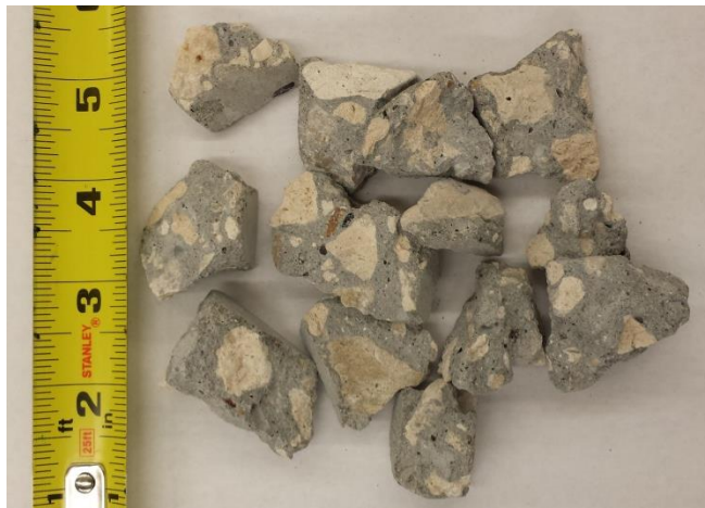
Figure 5.8: PCC specimen containing BA with particle size greater than 20 mm
