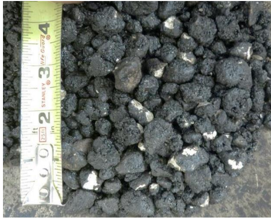
Figure 5.1: HMA specimen containing BA with particle size greater than 9.5 mm
