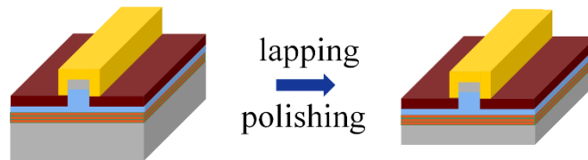
Figure 13: The wafer is lapped and polished to a thickness of \sim 150 \mu\text{m} before cleaving into individual devices from the device bar.
