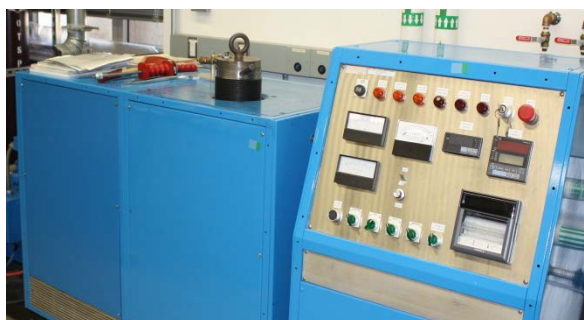
Figure 9: Hot Isostatic Press in the Optical Ceramics Laboratory at UCF manufactured by American Isostatic Presses and capable of 1800°C and 230MPa.
