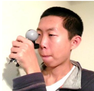
Fig. 56 Use an external reader to receive the data of eye pressure from the IC inside human eyes.
