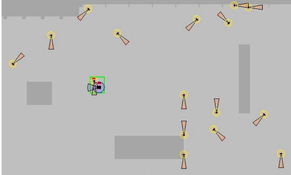
Figure 7.1: Scene from the recorded video with 20 crowd members (sparse crowd). The dark grey boxes are static obstacles. For each crowd participant we show the physical space, personal space and intended movement cone. Active micro-conflicts are indicated by rectangles surrounding the participants.
