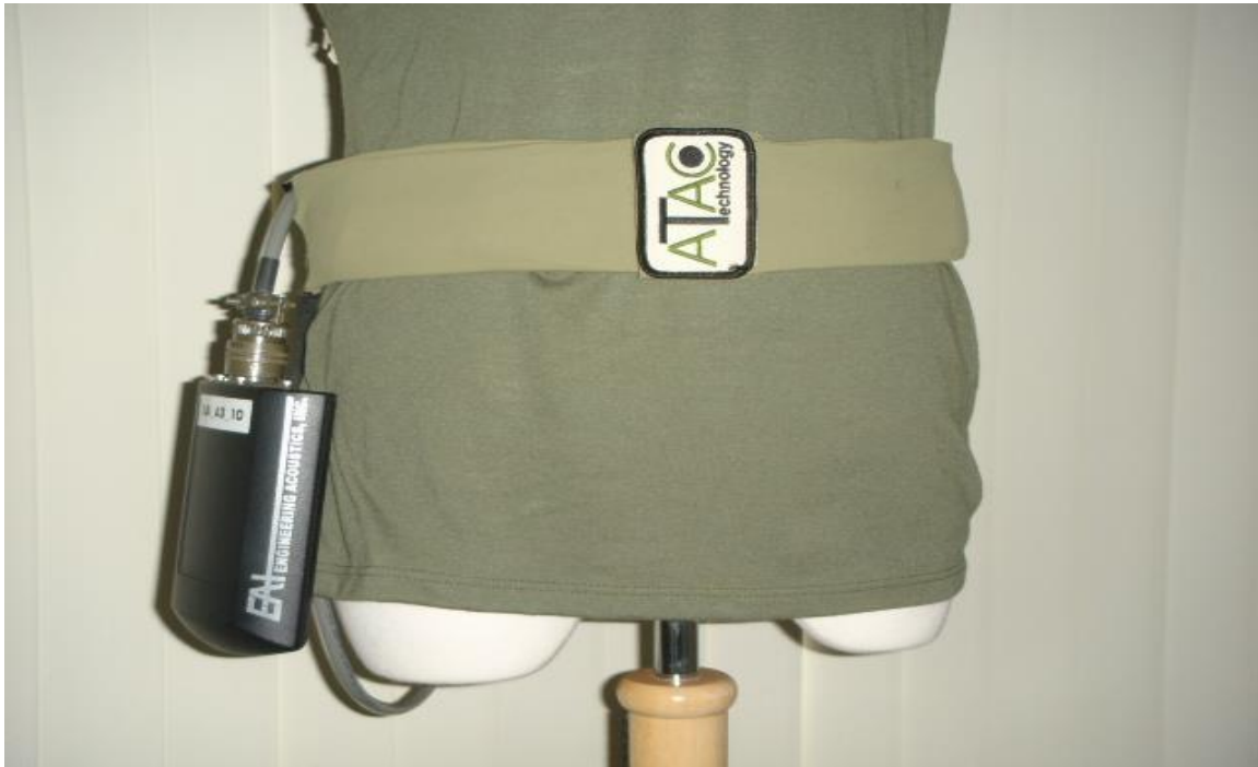
Figure 5. Tactile system developed by Engineering Acoustics Inc. Shown is an adjustable belt that contains twelve C-2 factors and the control unit.
