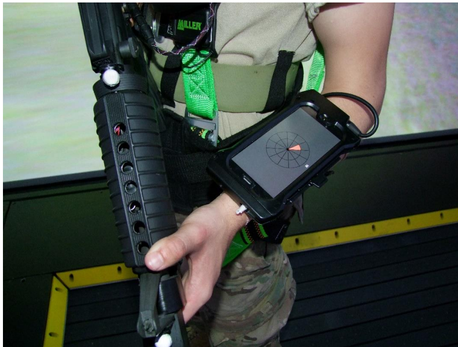
Figure 7. Samsung Galaxy S4 cell phone enclosed in a Juggernaut phone case. Shown on the display of the cell phone is a 10 o'clock, near cue.
