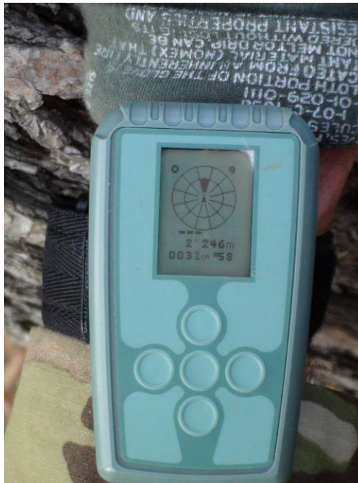
Figure 3. Visual display of the SWATS showing distance (in meters) and icon representing the azimuth location of an enemy shooter.
